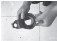
3. Put gasket seal in the Mechanical Tee.
