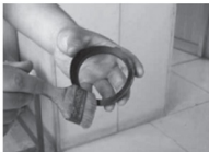
2. Spread lubricant on gasket ring.
